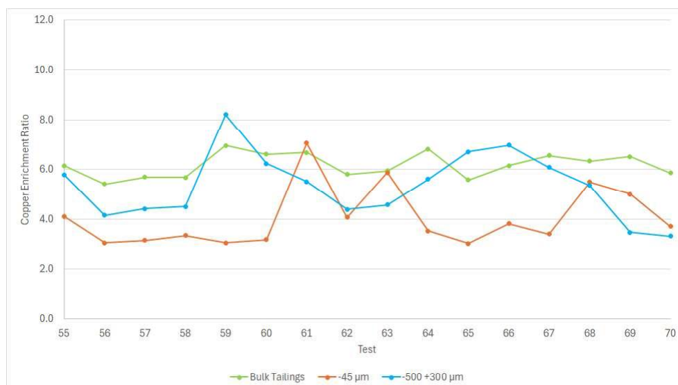
Figure 4 Pilot NovaCell™ copper enrichment ratio for bulk tailings, – 45 µm & – 500+300 µm material
