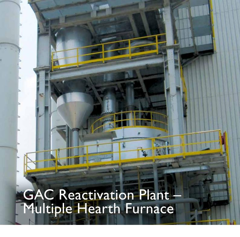
Jord Multiple Hearth Furnace's are used to effectively reactivate exhausted GAC from the decolourisation plant ready for reuse.
