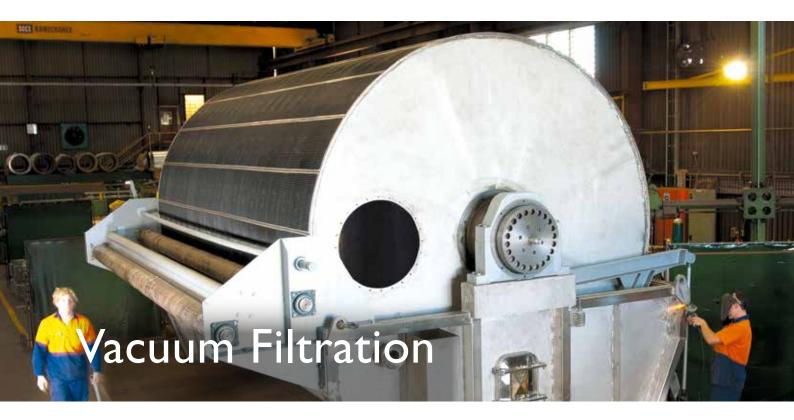
Jord's history with Rotary Drum Vacuum Filters (RDVF) dates back 45 years to its very first order, a cane mud filter for the Racecourse sugar mill in QLD. This order spawned an installation list of many hundred RDVF's across the globe, renowned for their longevity and superior design.
